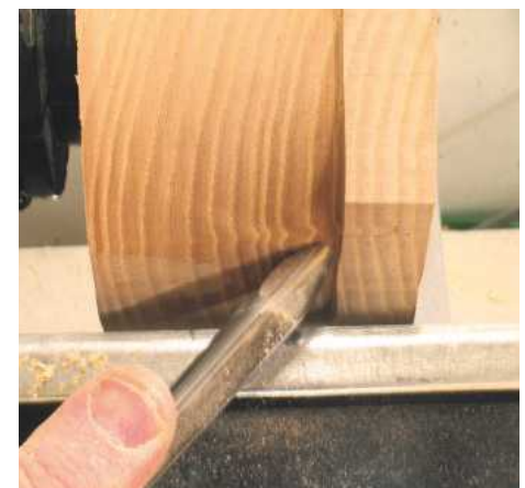
▲ Pic.3 If your lathe has the horsepower, you can take a large cut and make it round in one or two passes, even when the wood is cut into an octagon. Make sure the bevel of the tool is pointing in the direction of the cut
